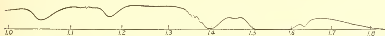
FIG. 3.—Energy transmission curve showing absorption spectrum of 5 cm. cell of liquid HCN at high dispersion. Slit width approx. 9\text{\AA} .
