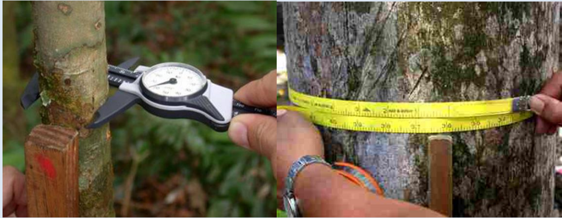
Figure 7.7. Measuring trunk diameter with calipers (left) and diameter tape (right).
