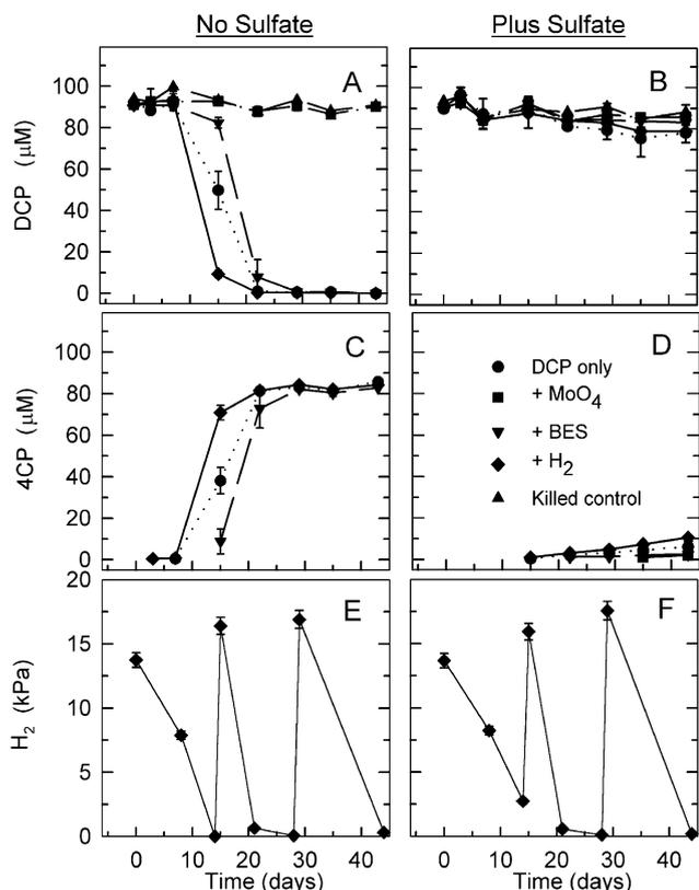
Fig. 1. DCP dechlorination in (A, C) sulfate-depleted and (B, D) sulfate-replete treatments of Experiment 2 and corresponding  $H_2$  concentration (E, F) in selected treatments. Data points are the average of duplicates  $\pm$  1 S.D.
