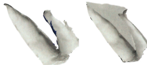
Figure 8. Left side: finished cast surface but empty mold area; Right side: restored mold.
