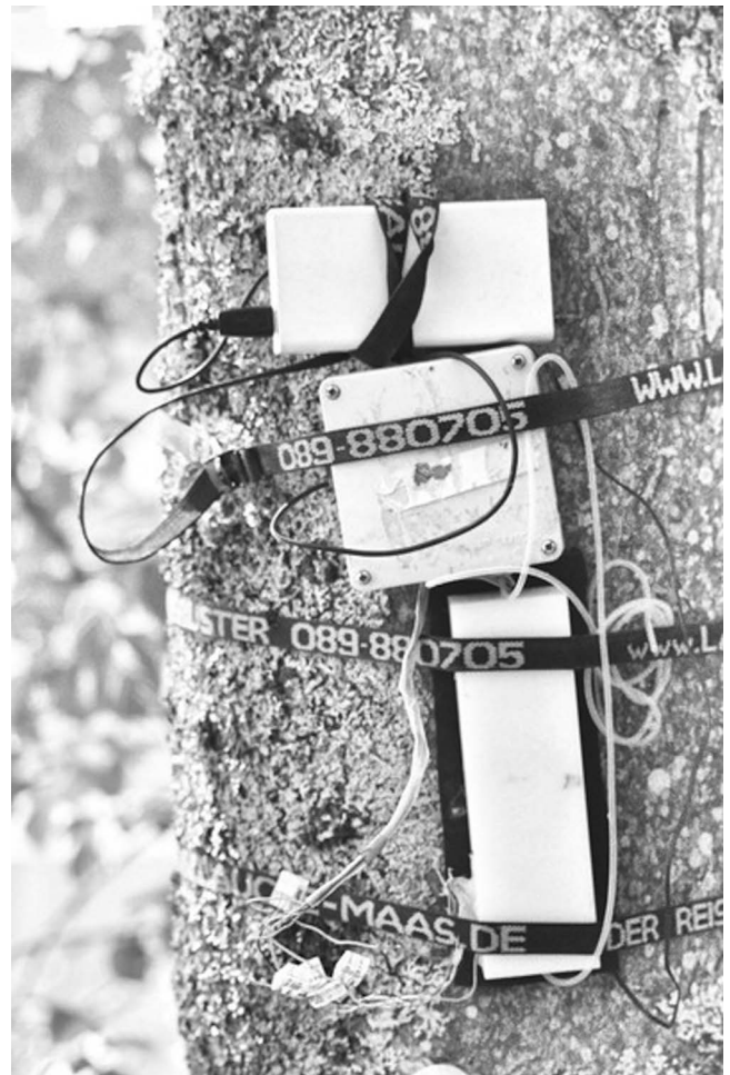
Figure 2. Photograph of the CDC system installed on an Acer pseudo-platanus tree during validation campaign with an Li-8100 system. On top is the power bank, in the middle the plastic box with the electronic components (microcontroller and pump) and below the chamber with the sensor inside.
