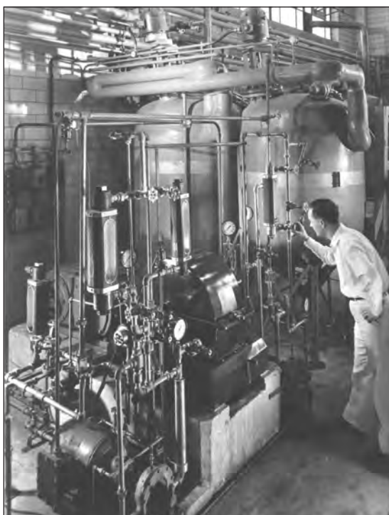
Deep tank fermentation, seen here at Abbott Laboratories in the 1940s, revolutionized the manufacture of antibiotics. Photograph Courtesy of the Kremers Reference Files [P39(g)].
