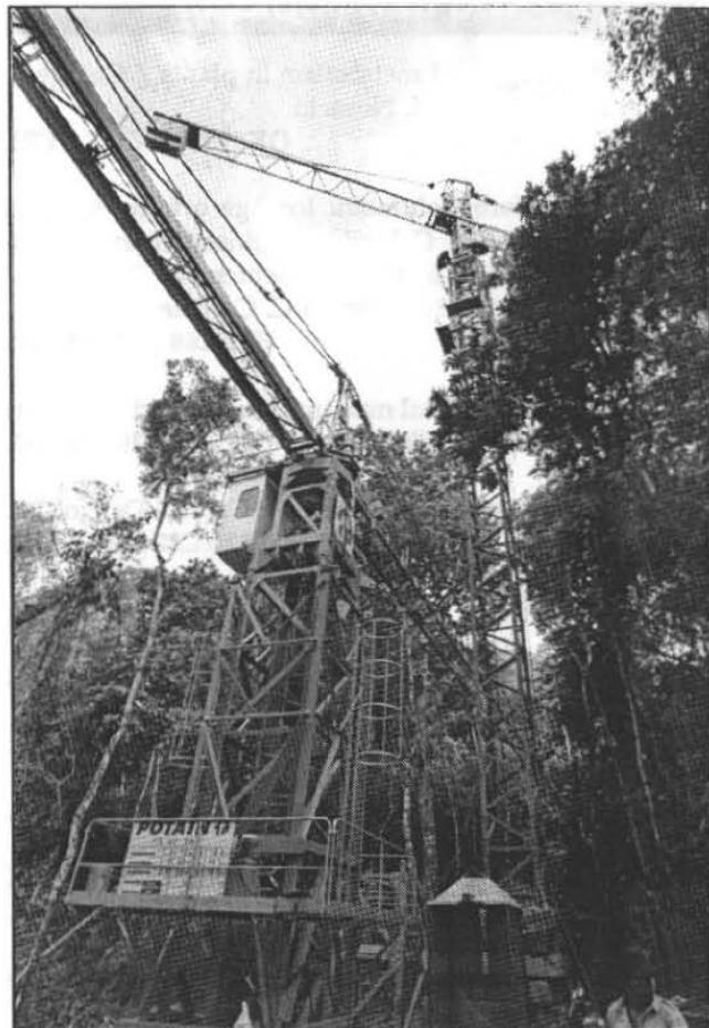
*This is the new Potain crane recently installed in the Parque Natural Metropolitano. This new crane will provide researchers access to a broader canopy area •••*
