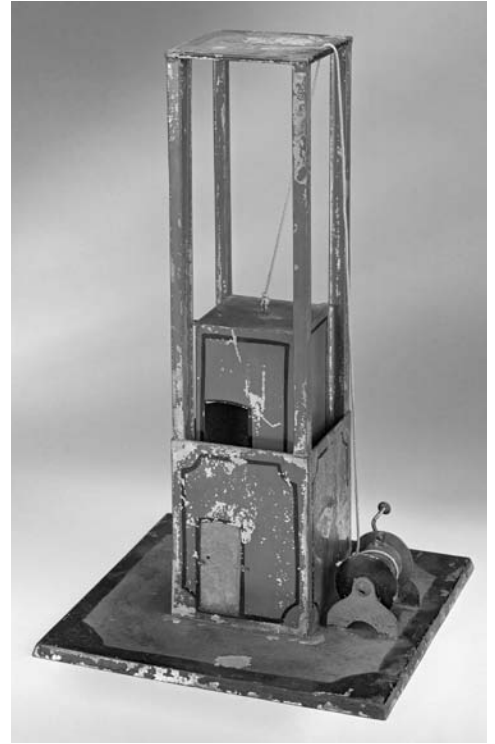
Patent No. 226,673. Charles R. Otis and Norton P. Otis. Elevator. April 20, 1880. (SI neg. 86-6159)
