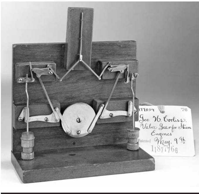
Patent No. 177,059. George H. Corliss. Valve Gear for Steam Engines. May 9, 1876. (SI neg. 86-6342)
