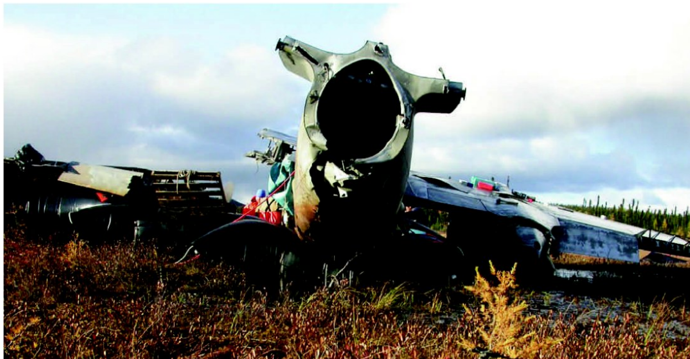
Figure 3: Tail section and port wing lifted by air bags. Note extensive damage to underbelly of fuselage and tail section (Deal)
