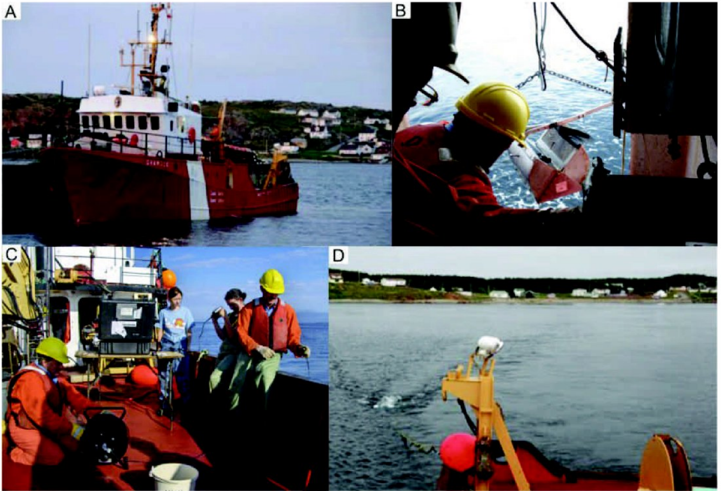
Figure 5: A) CCGS Shamook at Twillingate Harbour. B) Deployment of Van Veen grab for seabed sampling. C) Deployment of drop camera for seabed sampling. D) Deployment of IKB Seistec for sub-bottom profiling in Back Harbour (Westley et. al)
