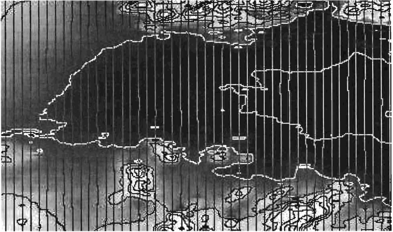
Plate 1. Geophysical survey flight lines overlaid on a DEM with 20-m contours marked. Note the wide contour spacing on the flatter areas. The survey lines are 400 m apart.
