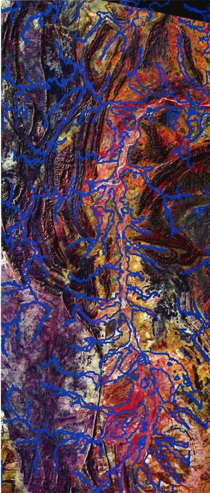
Plate 4. A Landsat TM image (copyright * Commonwealth of Australia, June 1988) overlaid with boundaries of the active flow area during a 50-year flood. Imagery is false color with TM band 2 = blue, TM band 3 = green and TM band 4 = red. Imagery provided by the Australian Centre for Remote Sensing, AUSLIG.
