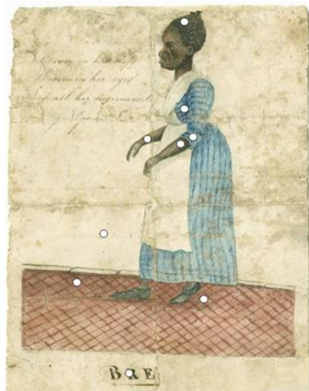
Fig. 1. Selected points for microfadeometry analysis on the 19.1 cm by 15.6 cm Miss Breme Jones watercolor.
