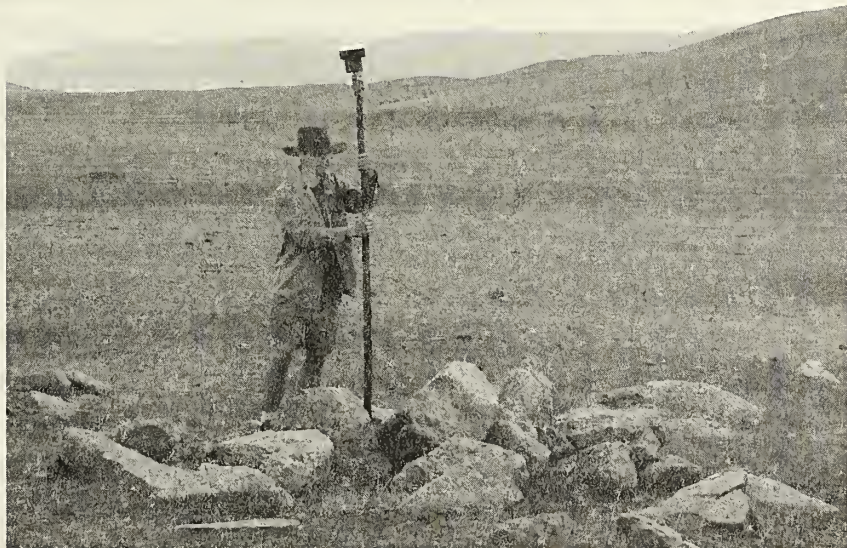
Figure 5.7. Matt Gallon recording points on Class II burial mound at Ulaan Tolgoi using the Ashtech/Magellan Locus GPS receiver (Rover). A central Base Station including a similar unit is placed permanently within a radius of 20 km. Using both receivers allows a precision of better than 3 cm.
