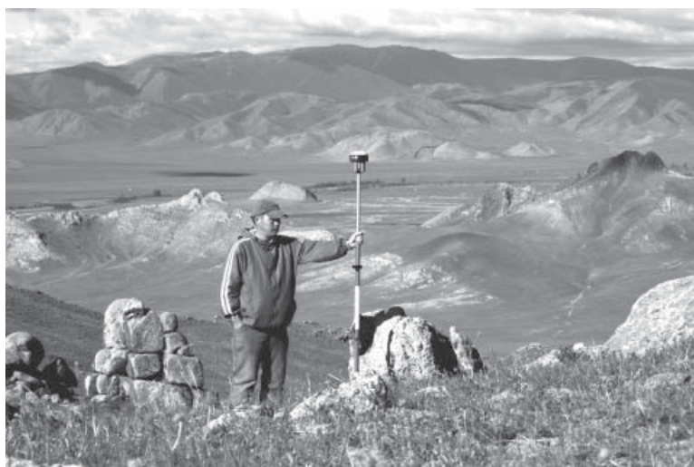
Fig. 3: Tsend Amgalantugs (Tugsuu) holding Ashtech/Magellan Rover unit used in surveying Bronze Age burial mounds.
