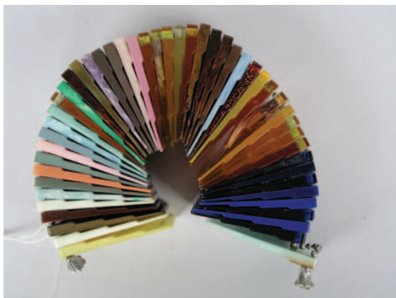
Figure 1 'Lumarith' (cellulose acetate) color samples kit manufactured in the late 1920s or 1930s. The sample kit consists of 49 coupons, each roughly 3.8 × 6.3 cm, looped on a 35 cm metal chain. Coupons have aged differently through time: some are in good condition, some samples exhibit signs of deterioration and some have undergone advanced deterioration.
