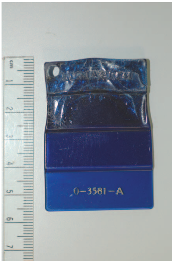
Figure 3 Example of a coupon (Coupon 9) in an advanced stage of deterioration.
