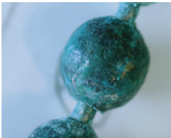
Figure 6 Green corrosion covers the surface of the metal ball (0.2 cm in diameter) from the nickel-plated metal chain. White flakes found in the corroded surface were identified as triphenyl phosphate by FT-Raman and XRD analysis.
