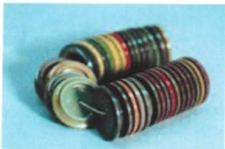
Fig 4. Bakelite color samples, 35 disks, each disk is 50 mm diameter and 8 mm deep. Late 1920's. Gift of Plastics Institute of America Thru: J. Harry Dubois. Smithsonian Institution.
