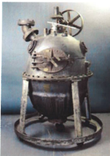
Fig. 2. Bakelizer, cast iron, ca. 1907. Gift of Union Carbide Corporation Thru: Dr. Nathan L. Zutty, President Specialty Chemicals Division and Warren M. Anderson, Chairman. Dimensions: 35" (W) 40" (D) 72" (H). Smithsonian Institution.
