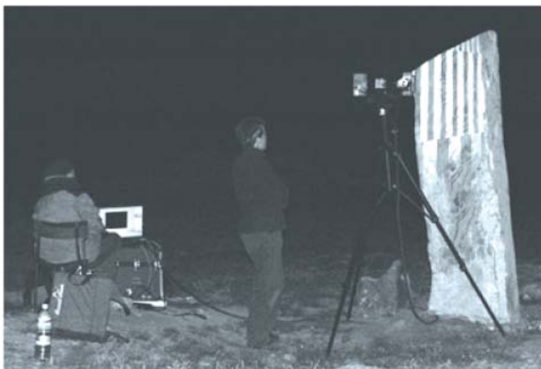
R. Beaubien (right) and L. Weber scan deer stone #2 at the site of Ushkiin Uver at night. Darkness increases the pattern definition of the structured light the scanner projects. (photo: V. Karas 2006)
