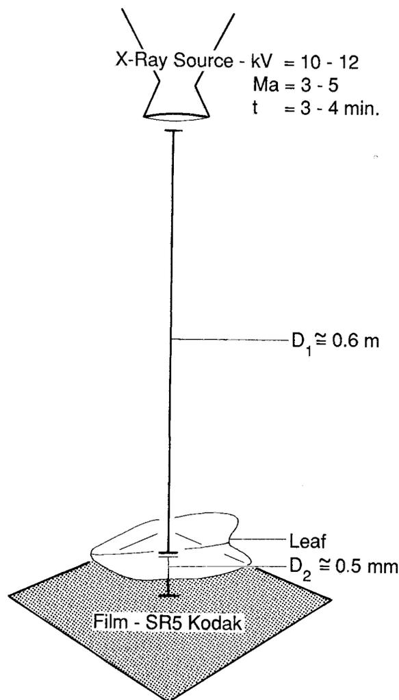
Fig. 1. Sketch of factors that can be varied in making leaf X-radiographs. kV = kilovoltage, Ma = milliamperage, t = exposure time,  $D_1$  = distance from X-ray to specimen, and  $D_2$  = distance from specimen to film.
