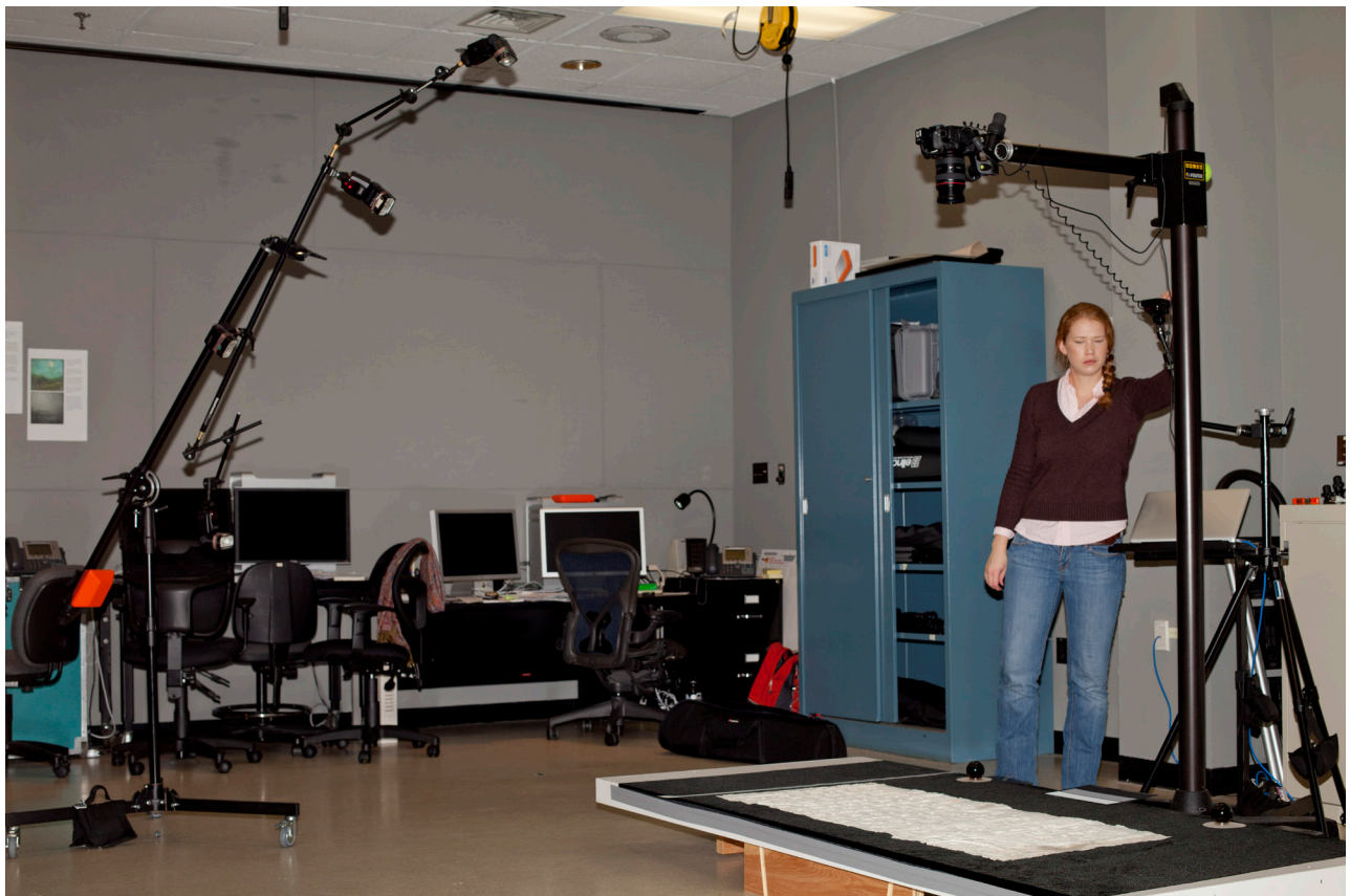
Figure 7 The Mantis in action. Webb triggering the flashes from a transmitter mounted on a tripod near the camera.
