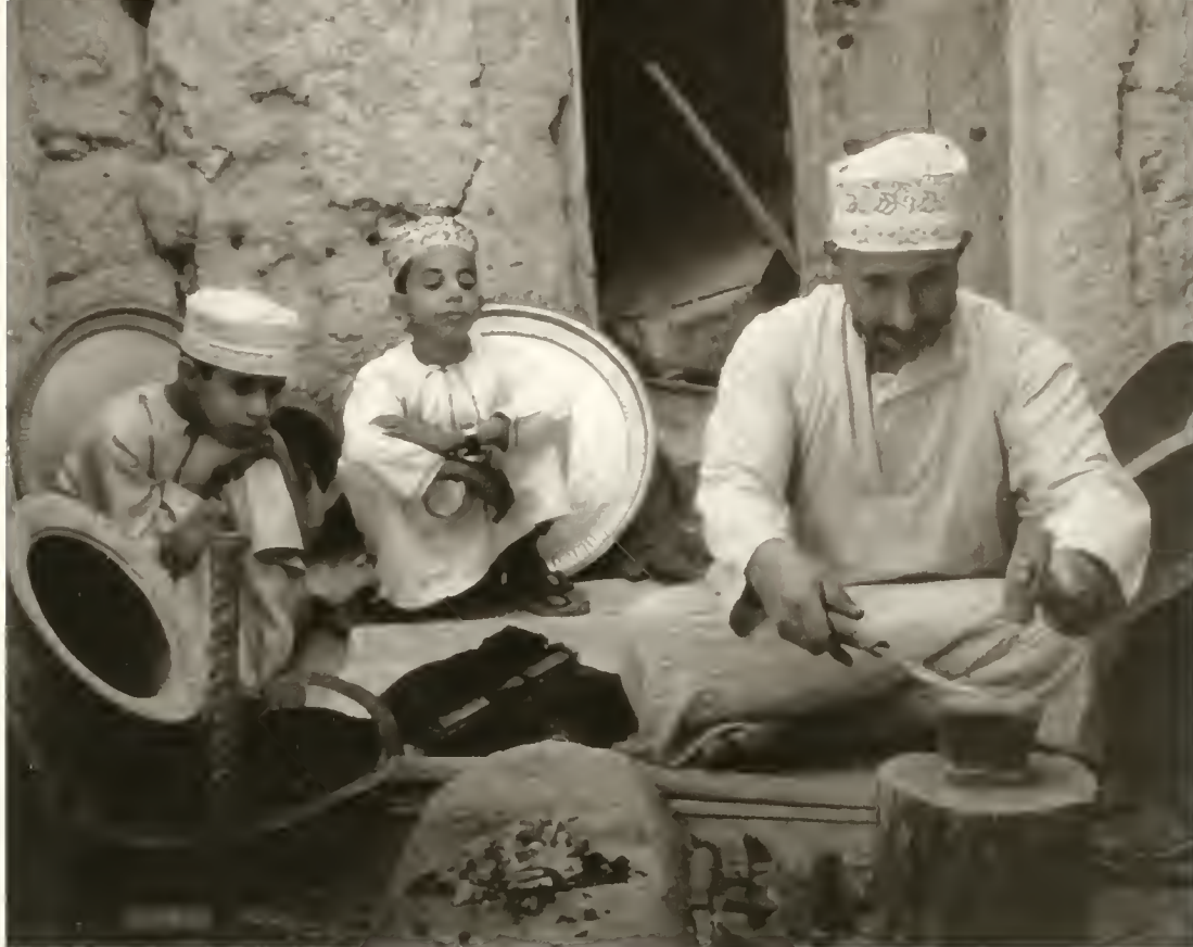
A Bahla blacksmith, assisted by his sons, employs hot-forging techniques to make a steel knife blade.
