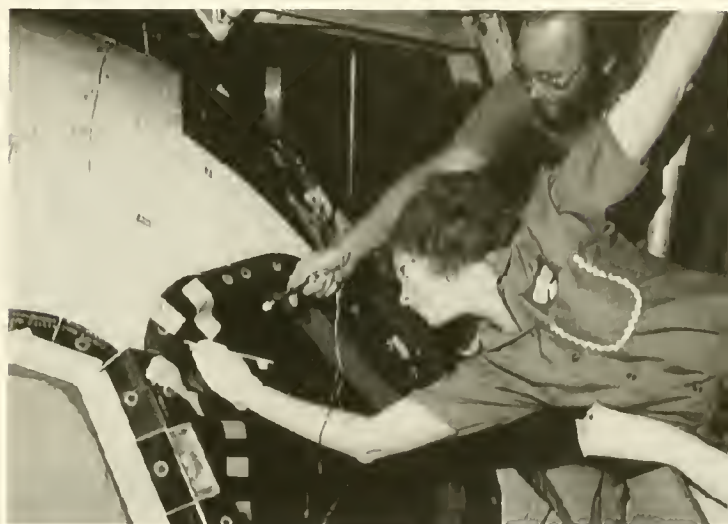
Technician Pat Klose leans over an edge in order to repair one of the protective thermal tiles on the Space Shuttle Columbia , prior to its fourth launch in 1982.
