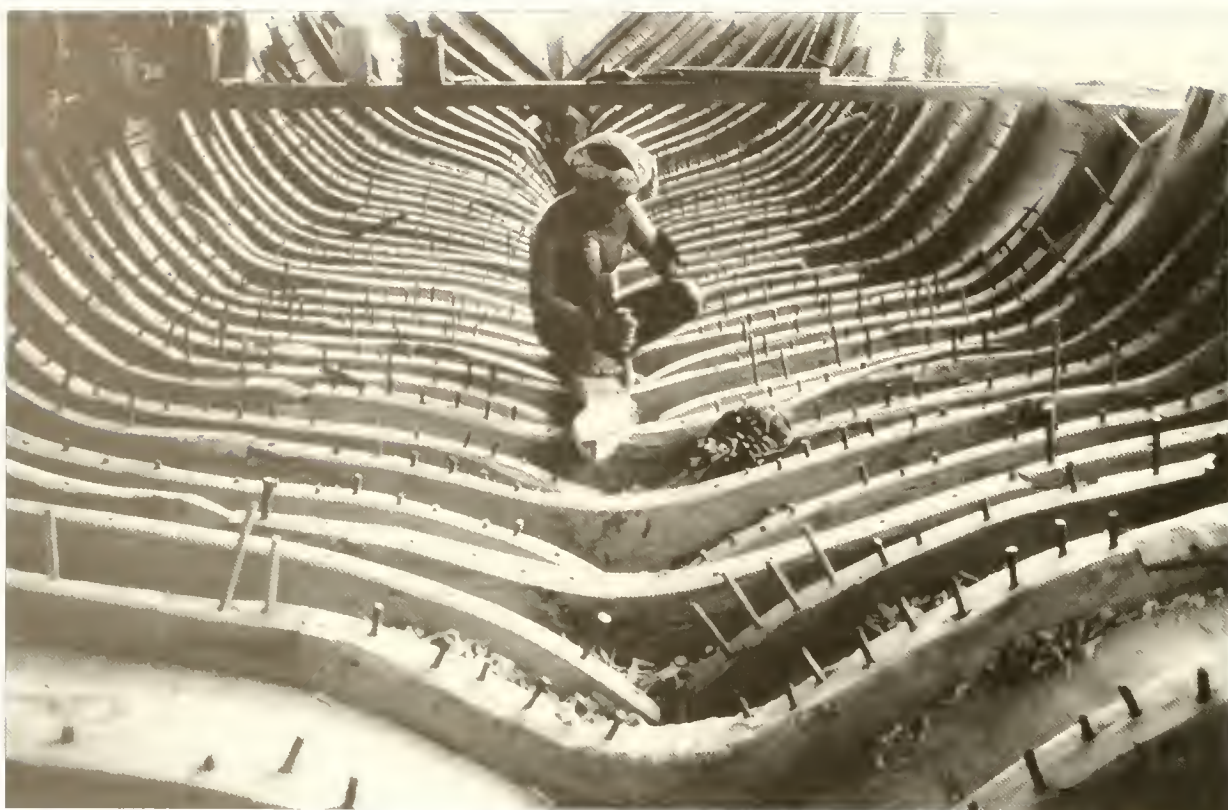
Above Sulawesi boatbuilders are renown throughout Indonesia. This boatbuilder near Majene, South Sulawesi, works with simple tools. The dourels are made of ironwood and the caulk of crushed coral and oil. The large ship he is building will carry cattle and passengers between Kalimantan (Borneo) and Sulawesi. Photo by Charles Zerner
