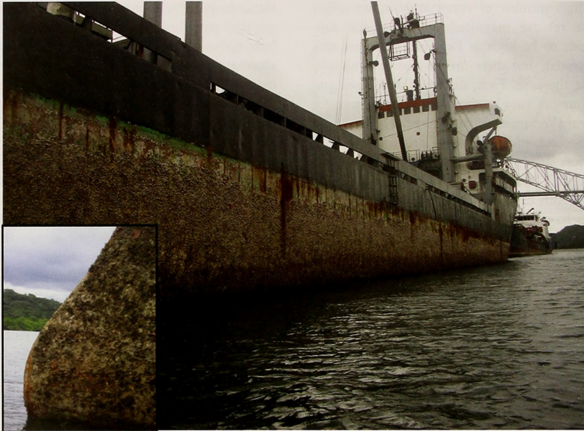
FIGURE 3. Photograph of a vessel hull upon arrival to Panama showing associated biofouling organisms. Inset: Close up of bow with barnacles.
