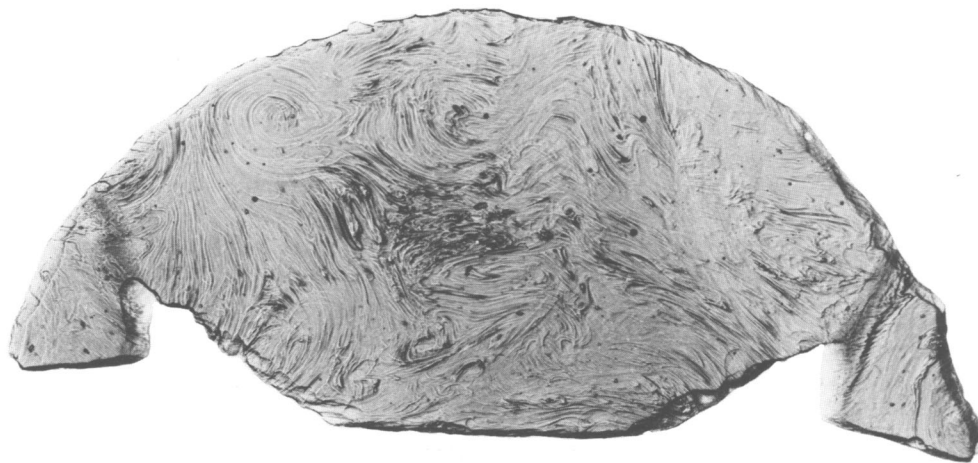
FIGURE 16.—Thin section of flanged australite button from Motpena, South Australia, showing flow structure and schlieren of differing refractive index.
