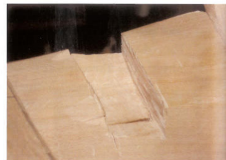
Figure 17 Rear seat rail dado for receiving the continuous back/seat slat.
