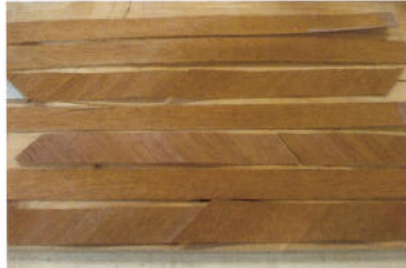
Figure 20 Laying out the veneers prior to laminating.
