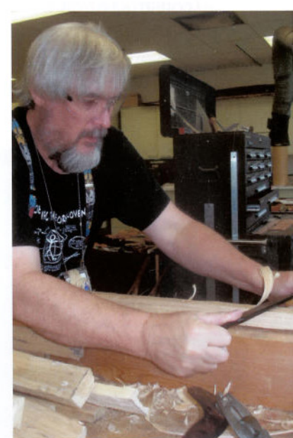
Figure 6 Stock was prepared for steam bending with a drawknife on a shaving beam, followed by spokeshaves and hand planes. Photo by Juliane Derry.
