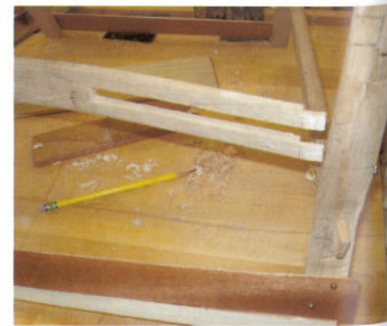
Figure 9 Tines were cut on the curved front stretcher after a tenon was cut on the full-sized element.
