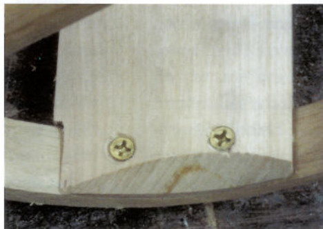
Figure 12 Gragg used screws and nails wherever two pieces intersected or were joined, such as these large screws from the underside of the front seat rail.
