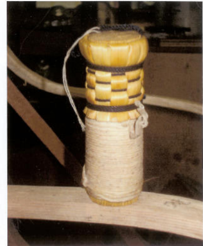
Figure 22 A corn straw burnisher is an ancient tool for final prepping of the surface before finishing.
