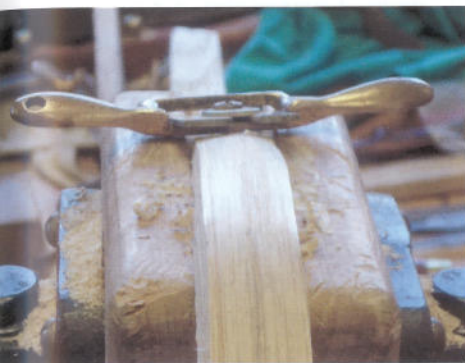
Figure 19 The ultimate elegance of the chair is in part due to relieving and rounding all the edges of the chair elements with a tiny spokeshave.
