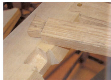
Figure 16 Front rail/seat slat half-blind dovetail, pre-assembly.
