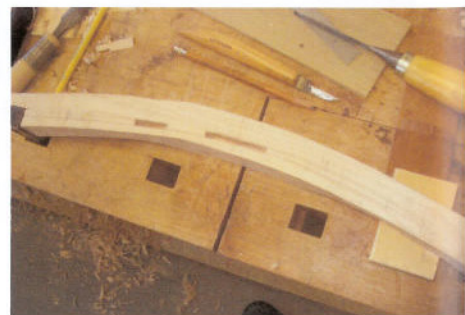
Figure 18 The narrow mortices for the splats are chopped into the crest rail.
