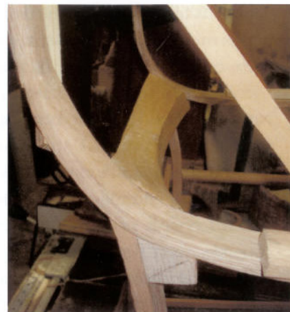
Figure 15 The rear seat rail, curved along all axes, was formed primarily with spokeshaves.
