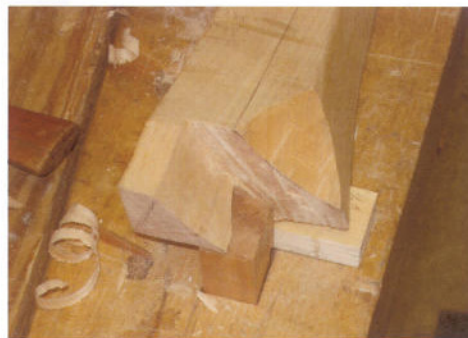
Figure 14 The joinery for the rear seat rail/leg junction was nearly impossible to get right the first time. It cannot be laid out precisely and must be sculpted to fit the spaces.
