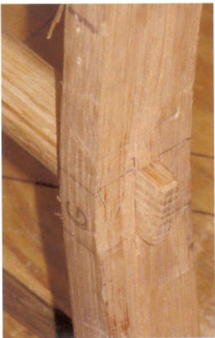
Figure 10 Through tenons were cut on the ends of the round chair rungs, and inserted through mortises in the legs.
