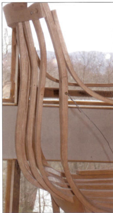
Figure 2 The slight variations of the back splat profiles allows the structure to act as an integrated leaf spring, each slight element reinforcing the others.
