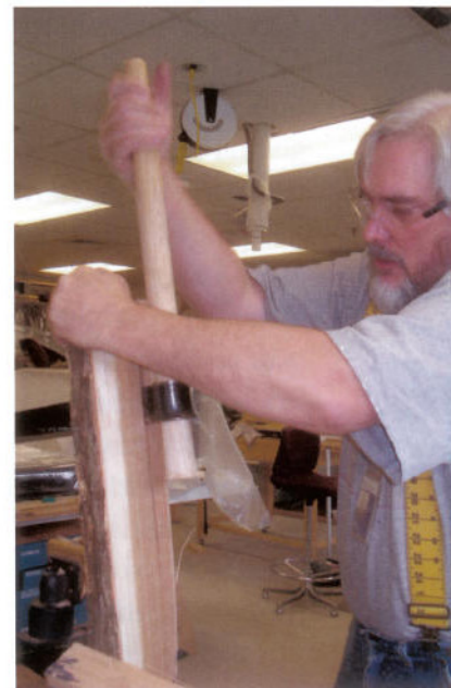
Figure 5 Stock was wrought with traditional tools and techniques; splitting the logs with mauls and wedges, followed by riving with a mallet and froe. Photo by Daniela Gross.
