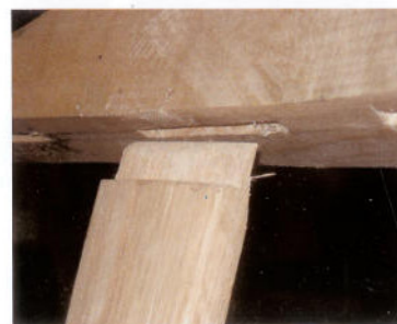
Figure 4 The crest rail is joined to the vertical back slats by delicate mortise and tenon joints.
