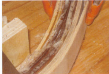
Figure 21 The assembled laminae, between two cauls and a plastic membrane.
