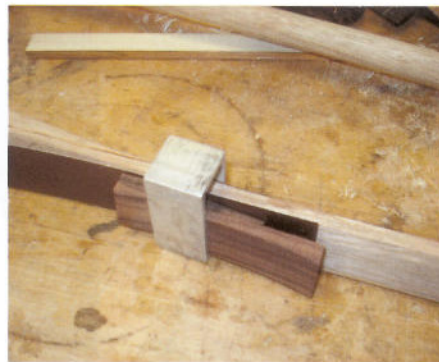
Figure 8 Clamping collars with pairs of tapered wedges hold the bending bands in place.
