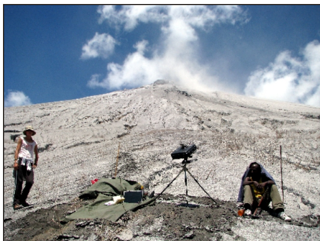
Figure 20. Mini-DOAS scan setup on 6 April 2008 on the W ascent route to Ol Doinyo Lengai. Courtesy of Maarten de Moor.
