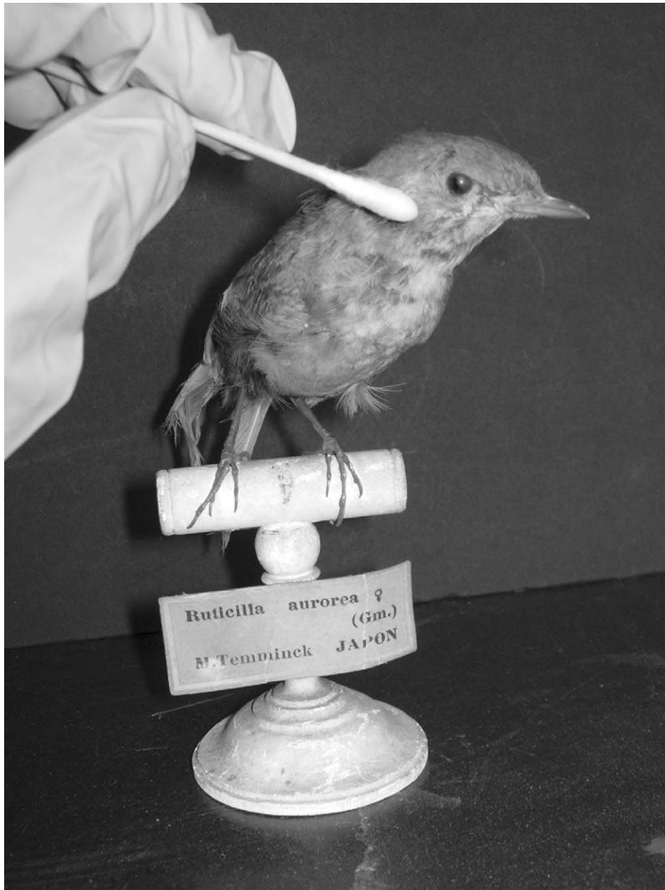
Figure 1. Rolling a cotton swab on a bird specimen for an Arsenic Spot Test at the Muséum National d'Histoire Naturelle, Paris.
