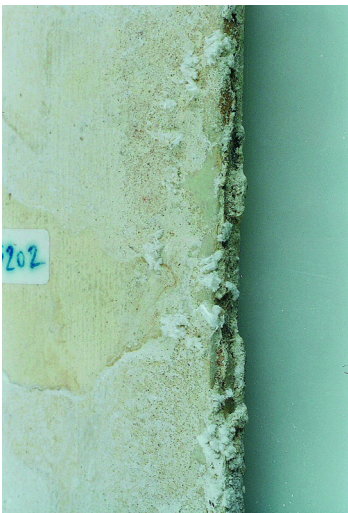
Figure 5. Back of tin-glazed tile (inv. 5202) with salt pustules
