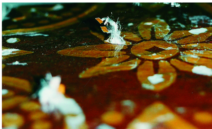
Figure 2. Long bundles of thecotrichite expelling glaze particles on Flemish tile (inv. 5545)
