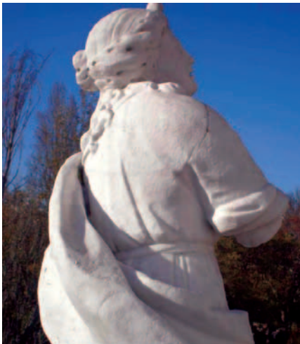
Fig. 3, a, b. Appearance of sandblasted marble sculptures. Micropitting of biocolonisation shows borders smoothed by the cleaning method.
