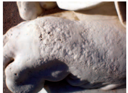
Fig. 3, a, b. Appearance of sandblasted marble sculptures. Micropitting of biocolonisation shows borders smoothed by the cleaning method.
