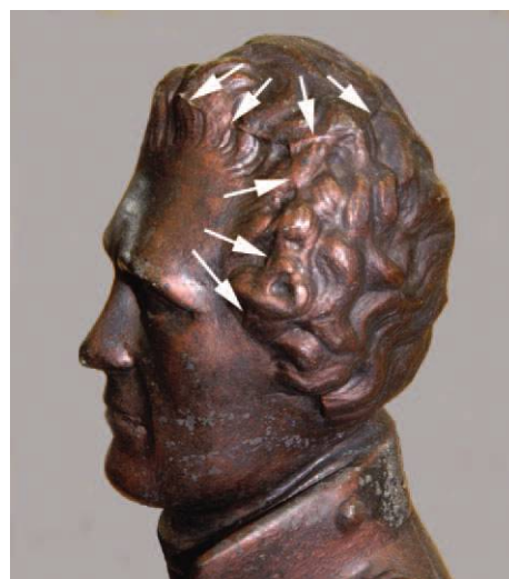
Fig. 14. Detail of Jackson's head, with arrows to mold-parting lines. (Smithsonian American Art Museum; photo, Carol Grissom.)
