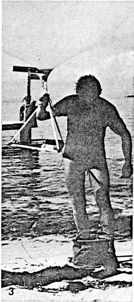
Figure 3 Tetrahedron frame with camera ready for use. A bucket holds the trigger cable and keeps the contact switch dry (photo: E. Kirsteuer).
