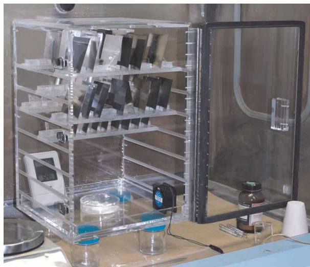
FIG. 1. Hydrogen-sulfide chamber containing silver coupons in the upper half. On the bottom of the chamber are the hygrometer (left), Petri dish containing barium sulfide (center), and fan (right).
