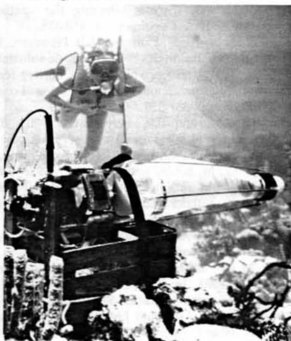
Figure 25. Stationary near-reef plankton sampler (hoplasa) installed on patch reef.
