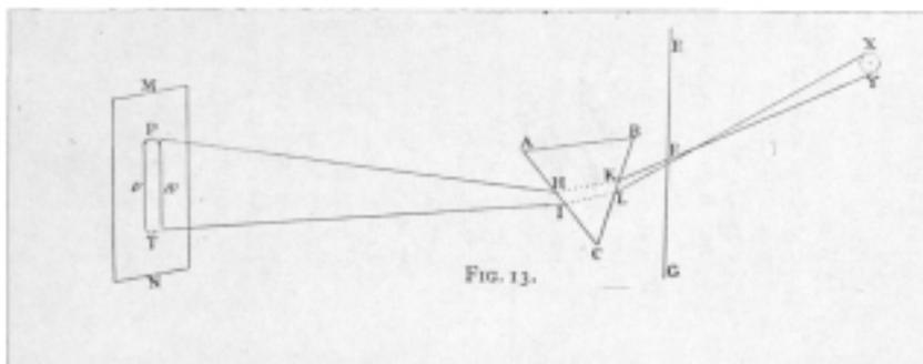
Figure 5. Newton's illustration—from the first edition (1704) of his *Opticks*—of the theorem that “The Light of the Sun consists of Rays differently Refrangible.” His arrangement of the prism and the resulting orientation of the solar spectrum—violet above and red below—became canonical and probably encouraged the terminology of “ultraviolet” and “infrared.” Courtesy Dibner Library, Smithsonian Institution Libraries.
