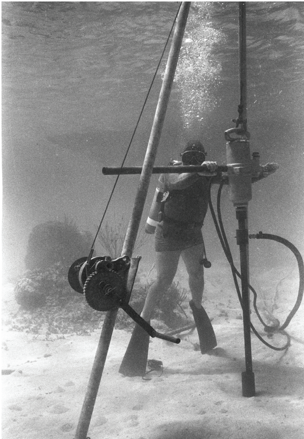
Figure 11. Drilling Core 7 in the shallow back reef of Tague Bay reef. Note the coral patches with surrounding sand.
