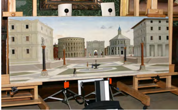
Figure 2: RTI set up for large panel painting: reference spheres at top, scale and color target below.
