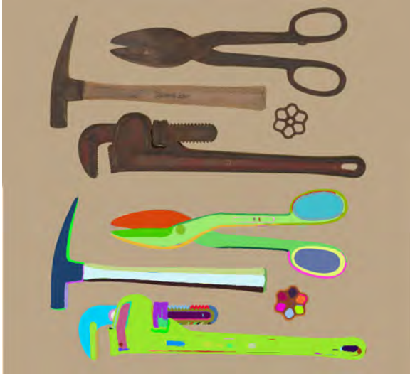
Figure 9: RGBN segmentation produced accurate results without visible color edges. The hammer has been segmented into multiple facets
