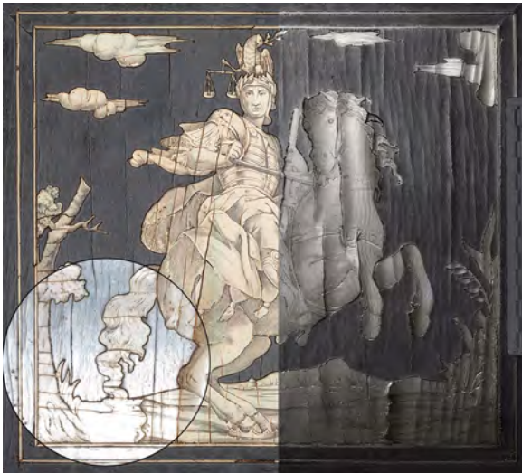
Figure 5: Detail of French polished ebony and ivory veneered door (approx. 30cm x 30cm). RTI image at left "illuminated" by source perpendicular to surface. At right, specular enhancement and raking angle shows surface deformation and Shreger lines in ivory. Inset circle at lower left is from an actual image processed for the RTI and shows high reflection from flash at 65°.
