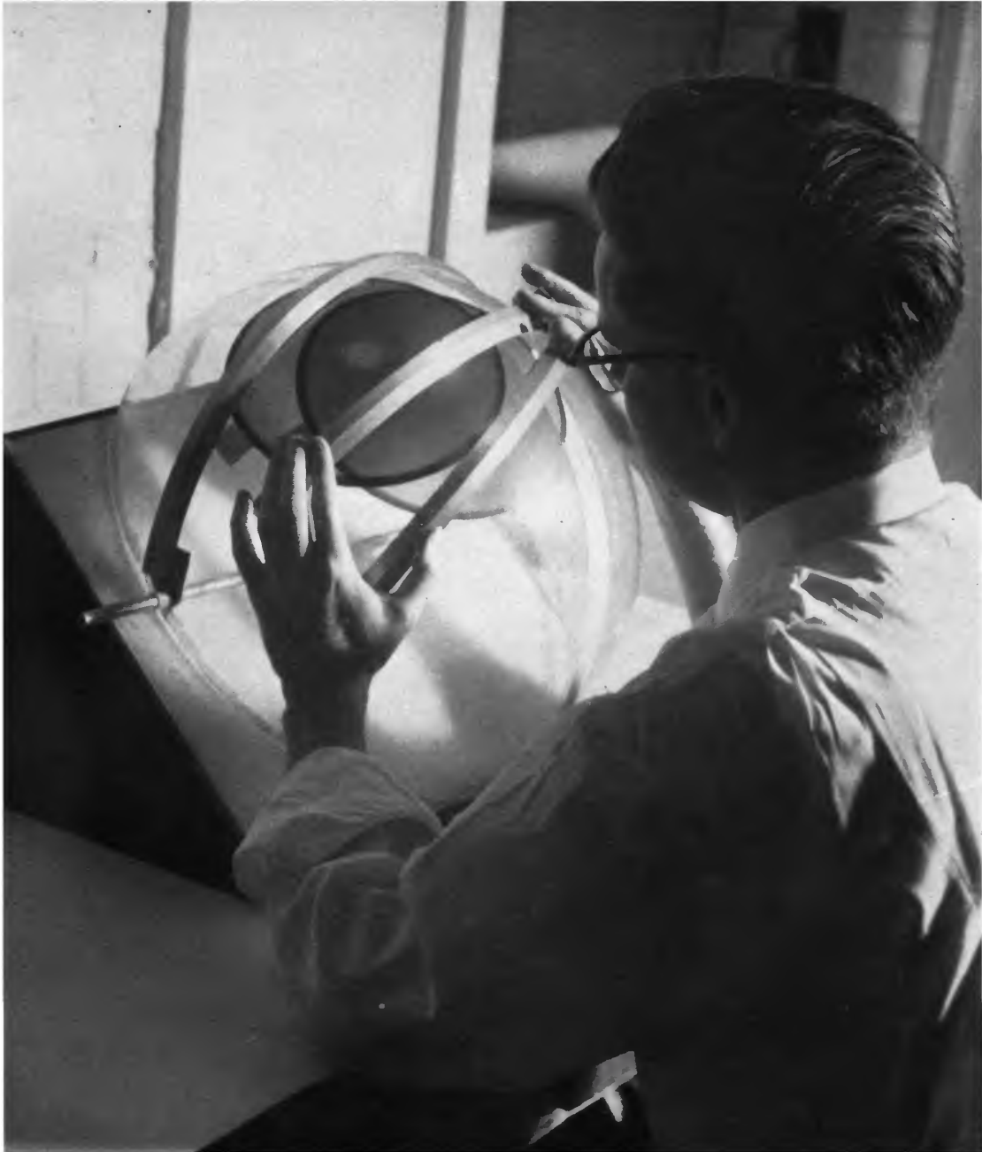
The transparent plotting globe. The declination scale pivots about the horizontal rod which passes through the globe at the celestial poles. The computer is positioning the curved rules to be coincident with the meteor image on each film. The juncture of the rulers (under the right hand) represents the meteor's radiant.
