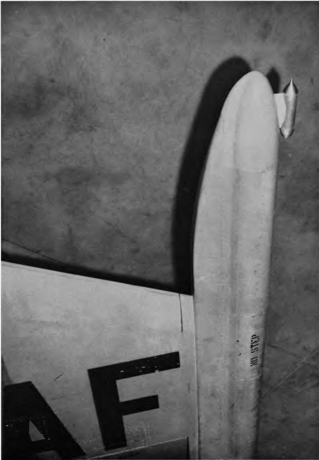
Wing tip of F-104A showing meteoritic dust collector in place. Photograph courtesy of NASA, Flight Research Center.
