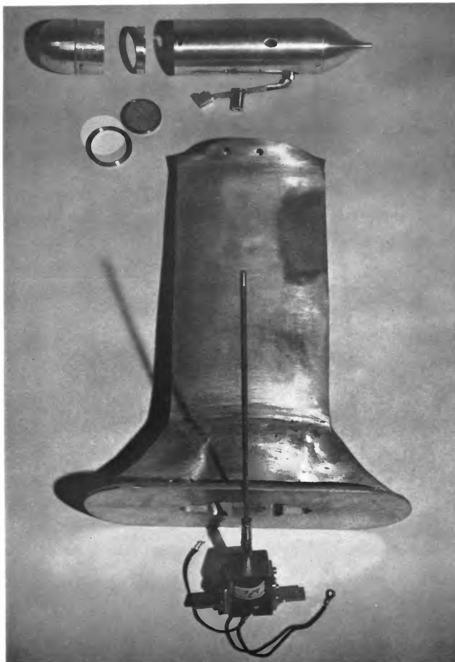
Unassembled parts of the second collector, which was carried by jet aircraft (B-52) out of Seattle, Wash.
