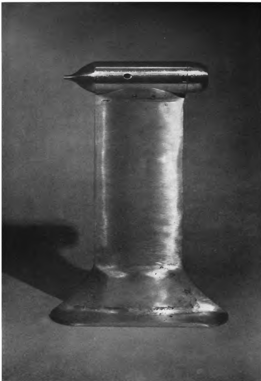
The second collector as assembled. The strut is 14 inches long.
