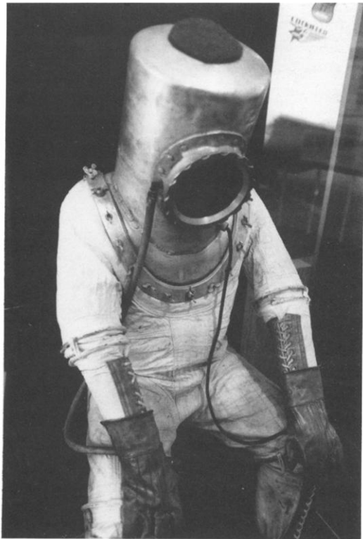
Fig. 1. Wiley Post's pressure suit, ca. 1934. As the world's first practical pressure suit, this was an important step on the road to space. Post wore this suit while setting a high-altitude, high-speed record in his plane, the Winnie Mae (March 1935).
