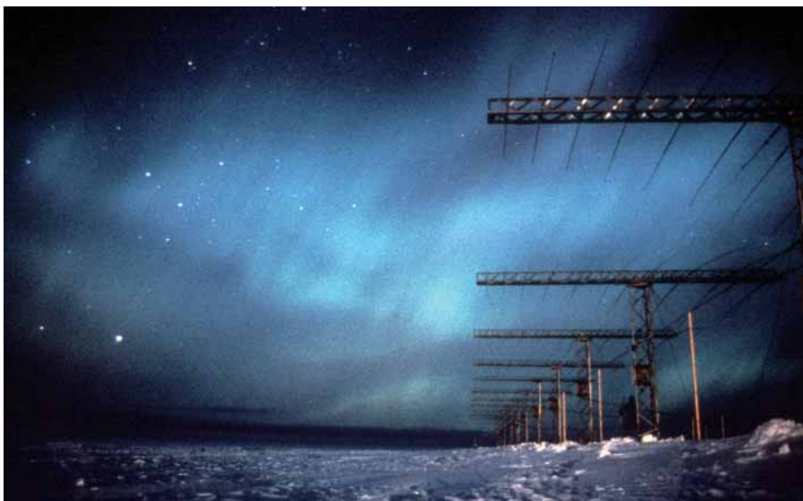
Aurora are the most obvious visual indication in the polar regions of the interaction of the Earth's magnetosphere and upper atmosphere. The polar regions offer unique platforms for studies of the atmosphere; the image illustrates the Super-DARN (Dual Auroral Radar Network) radar in Antarctica used for global ionospheric studies in conjunction with similar radar facilities in the Arctic.
