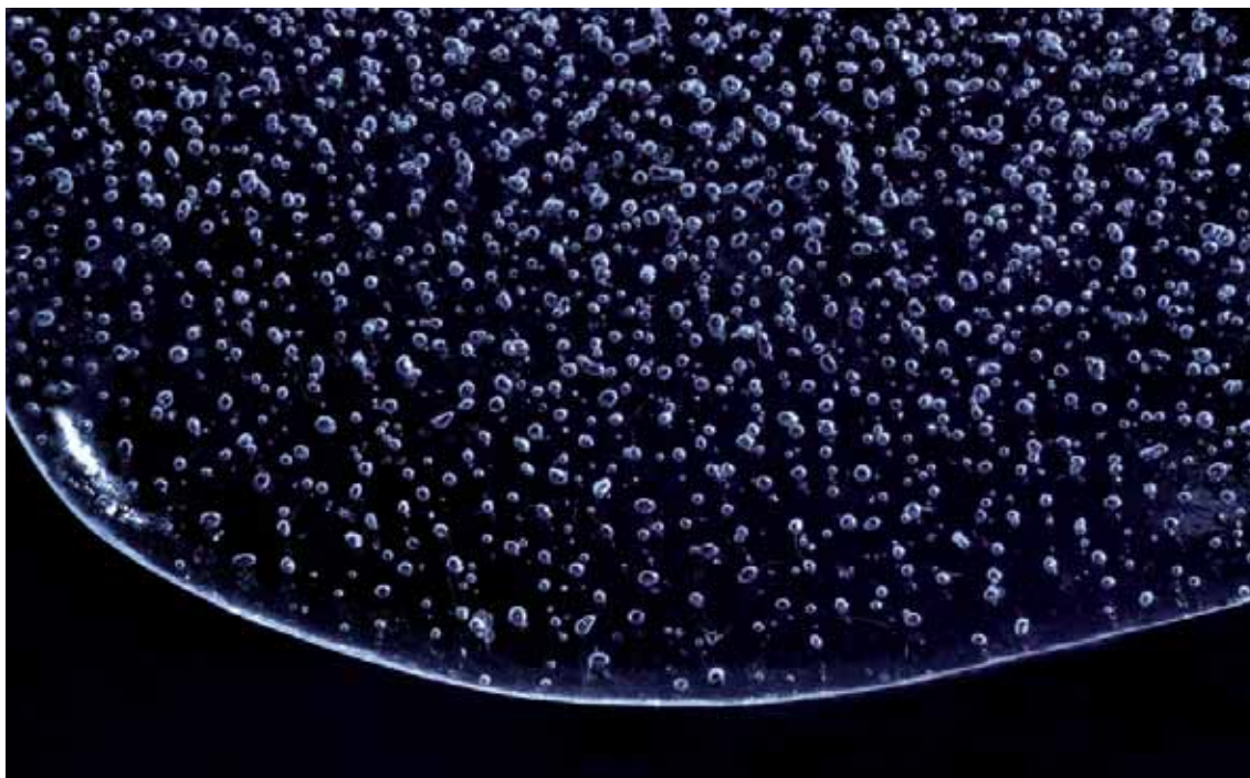
Glacial ice contains air trapped as minute bubbles. Analysis of the gas composition provides a sensitive historical record of past greenhouse gas composition, while isotopic analysis of the ice provides a temperature record.
