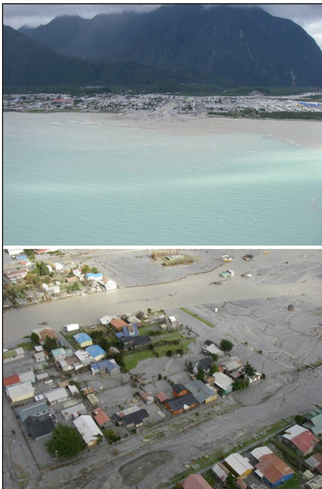
Figure 8. (top) Town of Chaitén overrun by lahars during mid-May to early June 2008. Lahars had begun to accumulate as a delta at the river mouth. Owing to sedimentation, the river (seen in background) had changed course and was then flowing through the town. The airport is on photo's right side between the town and the steep hill in background. (bottom) This closer view illustrates variable amounts of lahar damage affecting Chaitén town. This town was completely evacuated within several days of the eruption's onset. Photos by A.B. Lockhart, USGS.
