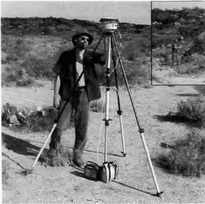
FIGURE 2. Components of the Trimble 4800 Differential Global Positioning System (DGPS). The base station collects data at a fixed location for the duration of the survey. The roving unit (inset) collects the survey points. Post-processing of data from both units provides the differentially corrected topographic data. Digital images taken by JRZ on 9/28/00; approved for publication by U.S. Army.
