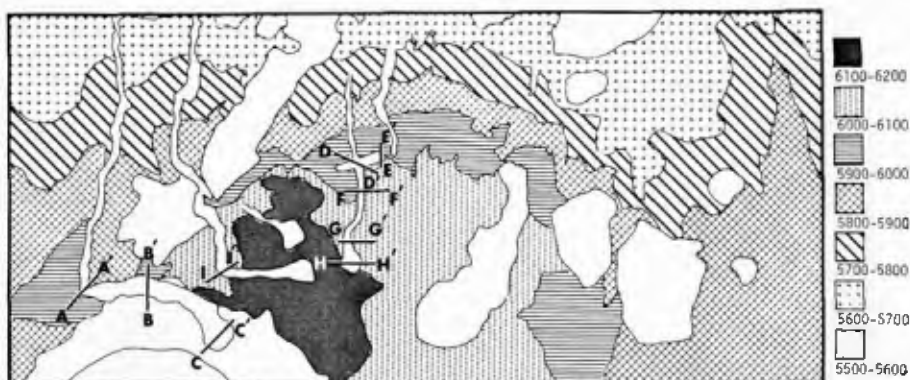
Fig. 2. Sketch showing topographic variation of the maria in the Prinz province summarized from the 1:250000 scale LTO. Elevations are in meters above an arbitrary datum of 1730000 m. Note the presence of a dome northeast of the crater Prinz. The rilles appear to originate on this dome. Lettered lines mark the traces of profiles across the rilles as shown in Figure 5.
