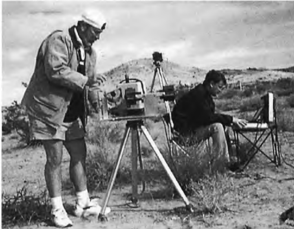
Figure 4. The thermal infrared spectrometer mounted on a tripod. The instrument was pointed by a field assistant (shown standing). Instrument functions and data collection are controlled by a laptop computer (operator seated).
