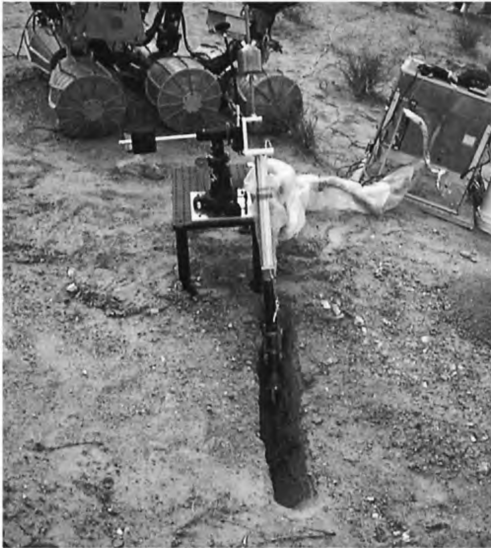
Figure 5. Robotic Arm Camera (RAC) imaging the walls of a trench. The RAC model is mounted on a tripod and positioned by an operator in the field. The control electronics are mounted in the equipment rack on the right side behind the tripod. Marsokhod is behind the RAC tripod bench.
