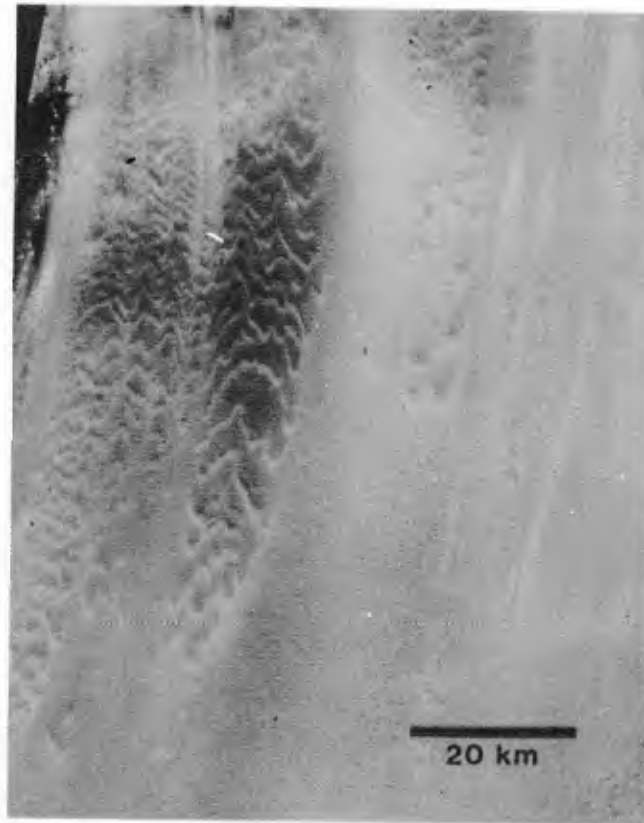
Figure 9. Chevron-shaped patterns at the northern edge of the Selima Sand Sheet. This near-infrared Landsat MSS image has been geometrically corrected and stretched to emphasize the patterns. Transverse high-frequency pattern in the lower part of this image are giant ripples reported by Breed et al. , 1987.
