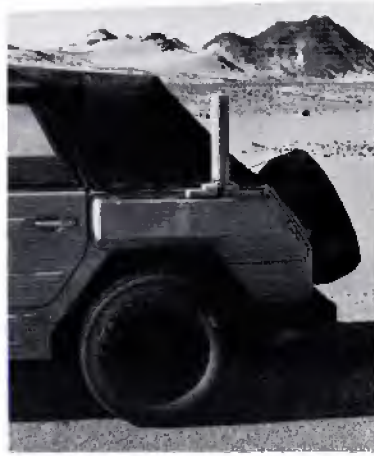
Figure 3.3 Nimbus-6 RAMS antenna mounted on rear of Volkswagen Type 181 desert vehicle.
