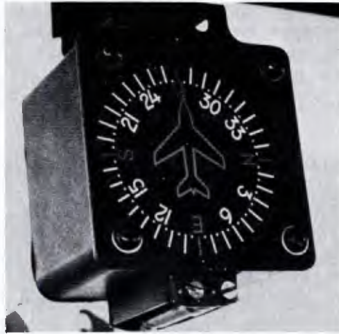
Figure 3.2 Vertical card compass mounted on windshield of Volkswagen Type 181 desert vehicle.
