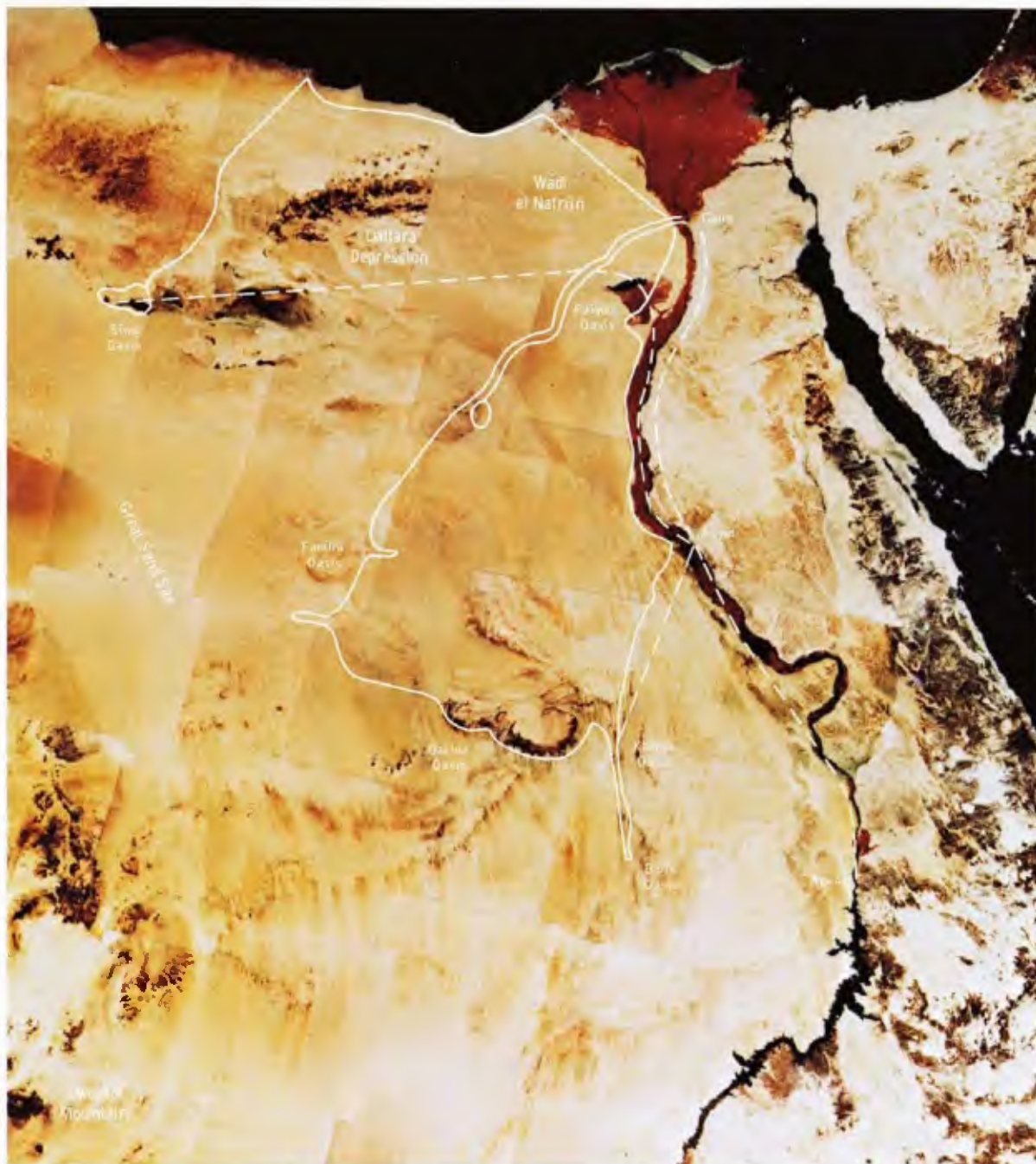
FIGURE 2.—Mosaic of false-color Landsat images of Egypt showing color variations in the exposed rock and soil. The tracks of field excursions in the Western Desert are shown with solid lines. The dashed lines indicate the paths of visual observation overflights at 1 to 2 km altitude.
