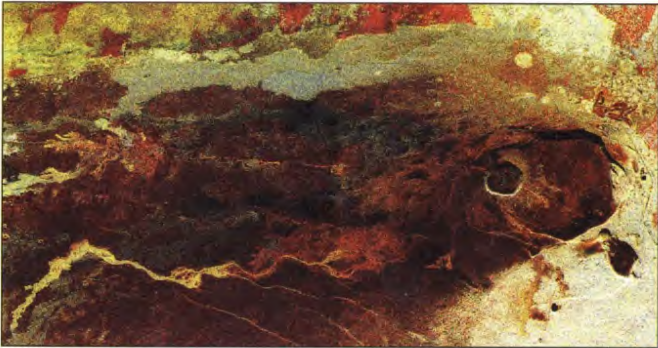
Plate 1. Radar image of Kilauea Caldera and Kau Desert study area. The 5.7-, 24-, and 68-cm HV echoes are coded as red, green, and blue channels, respectively. Image has been geometrically corrected to 10-m ground pixels. Image width 18 km. A'a flows appear as bright yellow or white, smooth pahoehoe surfaces are dark red, and vegetation near the caldera is white.
