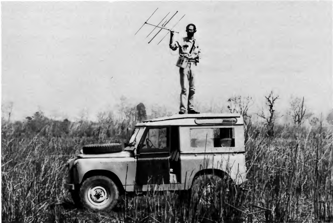
FIGURE 15.—Directional antenna attached to receiver used to electronically search an area for signals from radio-collared animals.
