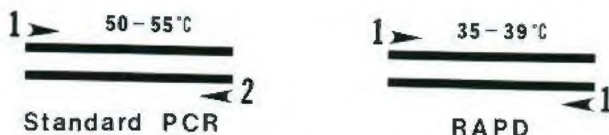
FIG. 1. Schematic showing the use of two primers of common length 18–25 bases in standard PCR versus the use of a single primer of common length 9–11 bases in RAPD reactions.
